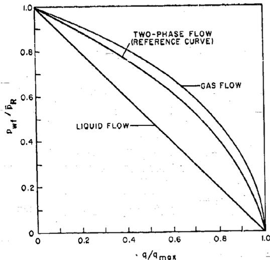
Fig. 8—Comparison of IPR's for liquid flow, gas flow and two-phase flow.
