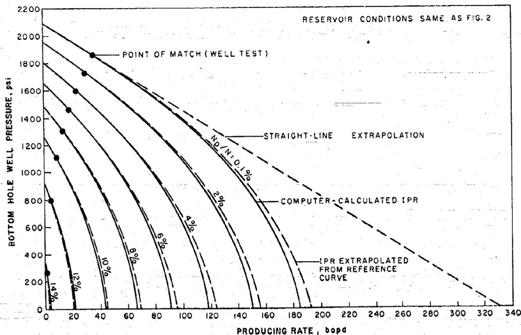
Fig. 7—Deviations when IPR's are predicted by reference curve from well tests at low drawdowns.
