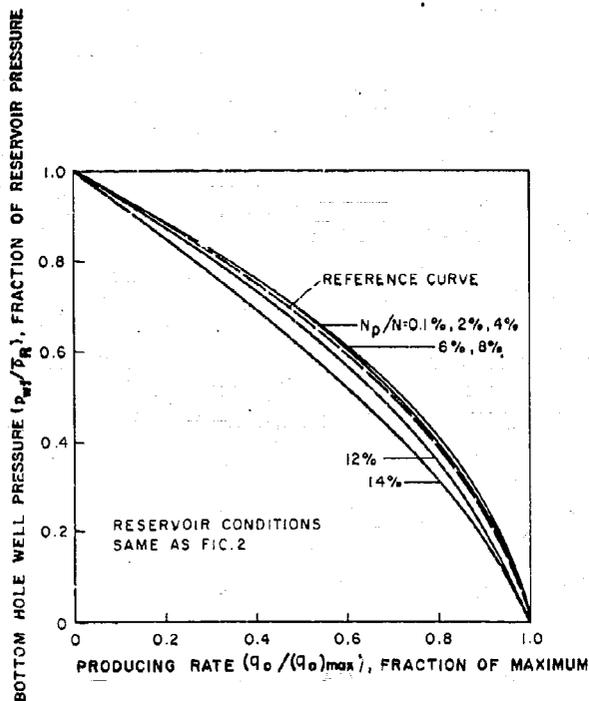
Fig. 6—Comparison of reference curve with computer-calculated IPR curves.
