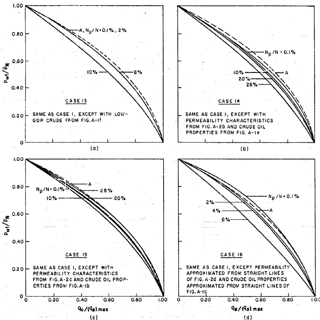
Fig. 14—Calculated dimensionless IPR curves.
