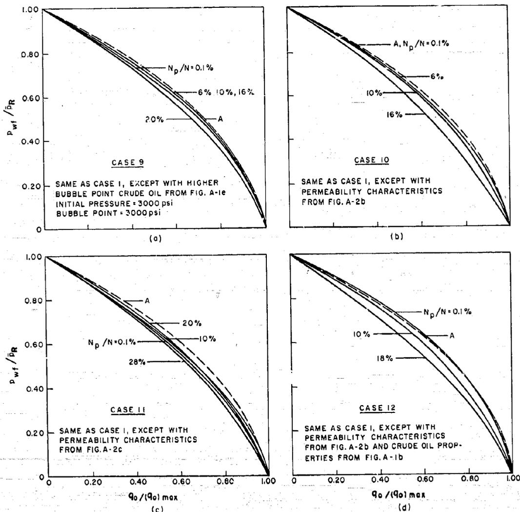
Fig. 13—Calculated dimensionless IPR curves.
