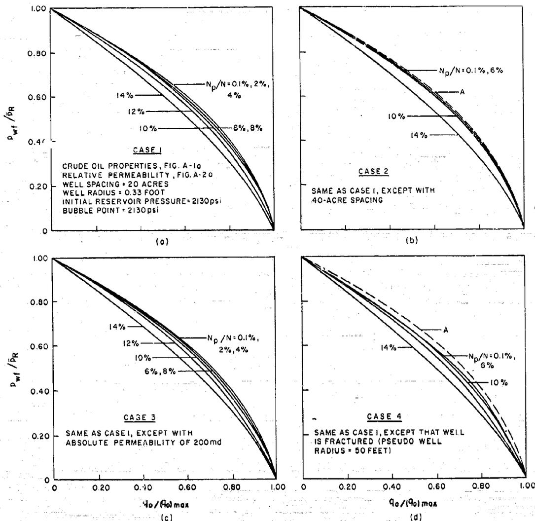
Fig. 11—Calculated dimensionless IPR curves.
