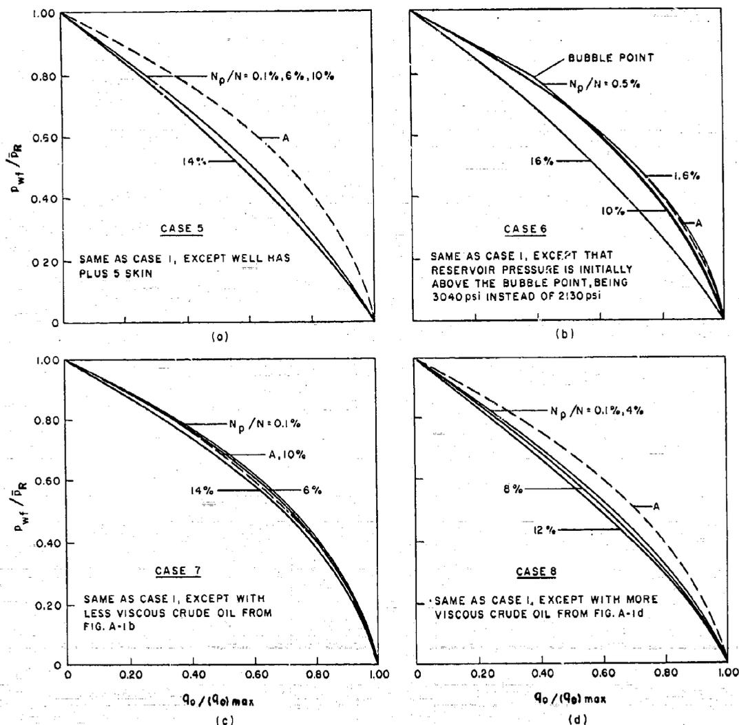
Fig. 12—Calculated dimensionless IPR curves.
