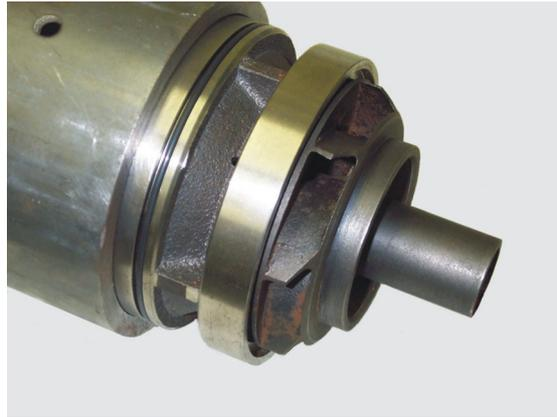
Figure 5 – A Pump Stage of the Pump
