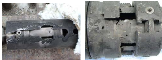
Figure 13. Corroded tubing patches
