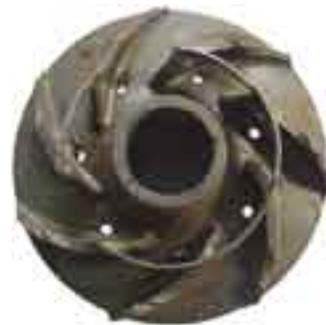
**Figure 3:** Severely worn impeller, subjected to pumping solids, observed in a pump teardown inspection.
