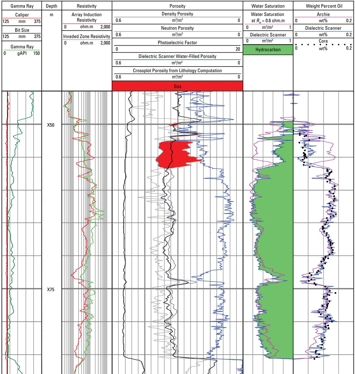
In Well 1, the varying formation water resistivity produced discrepancies in the conventional analysis based on the Archie equation, leading to a pessimistically high calculation of water saturation (Track 4). The weight percent bitumen calculated from Dielectric Scanner service's measurements is salinity independent and shows excellent agreement to core analysis results (Track 5).
