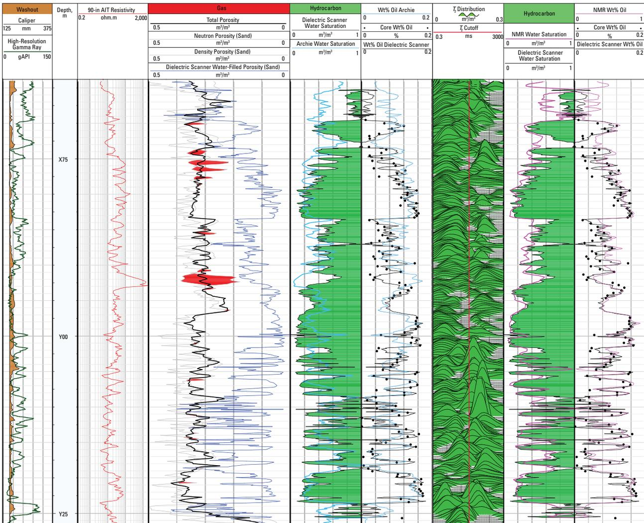
In Well 2, water saturation and hydrocarbon volume calculated from salinity-insensitive Dielectric Scanner service's measurements provide higher resolution, more accurate answers than those derived from the Archie equation or NMR data.
