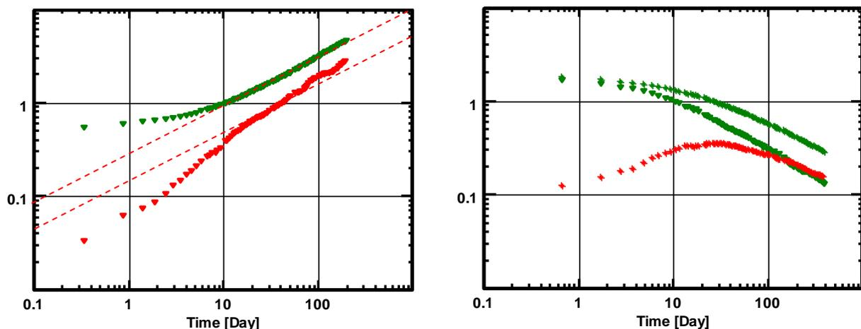
The data were analyzed and matched using (1) a square root plot defining a single equivalent fracture, (2) an analytical model for fractured horizontal well and (3) our numerical fractured horizontal well model using nonlinear (NL) diffusion. The history plot below shows that all
