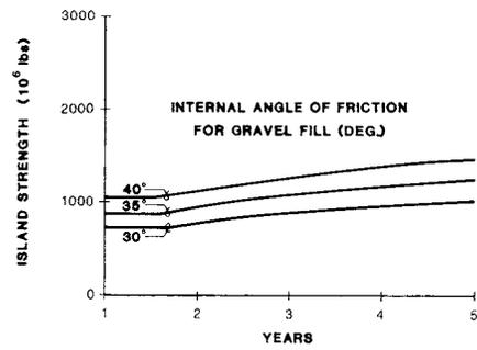
Fig. 8 ISLAND STRENGTH vs FRICTION ANGLE OF GRAVEL FILL
