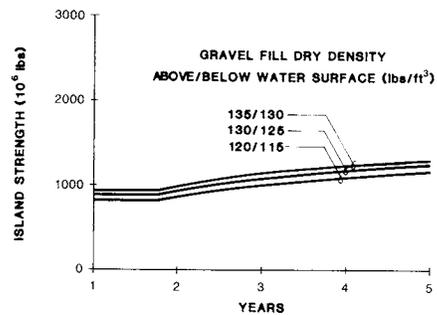
Fig. 12 ISLAND STRENGTH vs GRAVEL FILL DRY DENSITY
