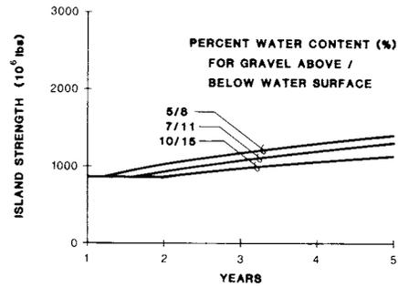
Fig. 10 ISLAND STRENGTH vs GRAVEL FILL WATER CONTENT
