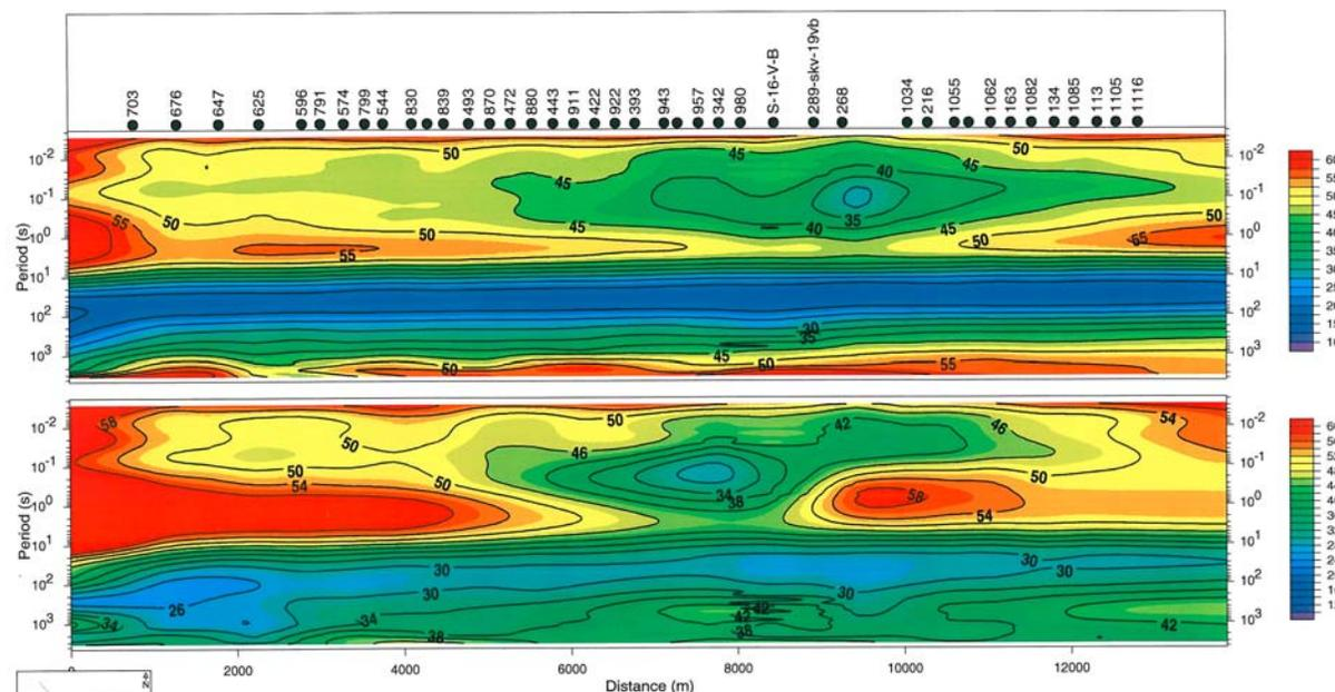
Figure 6: Impedance phase pseudo-section along profile P52.
