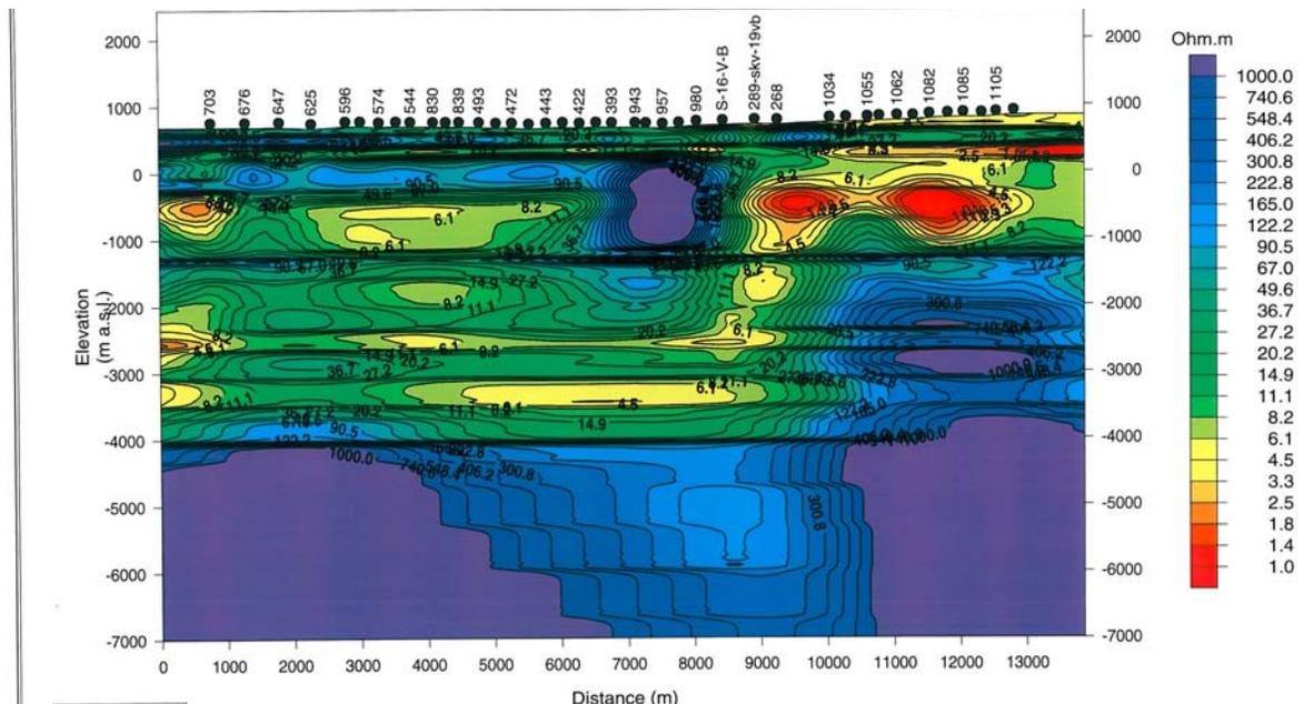
**Figure 7:**Results of 2-D inversion along profile P52.
