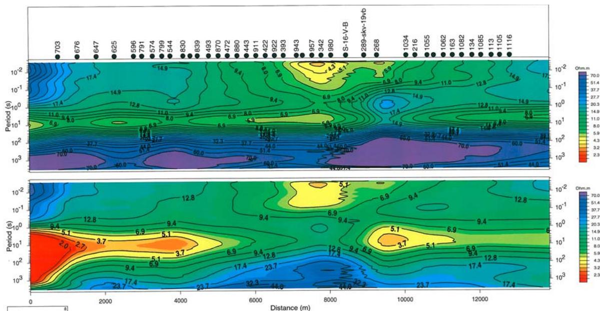
Figure 5: TE (top) and TM resistivity pseudo-section along profile P52.
