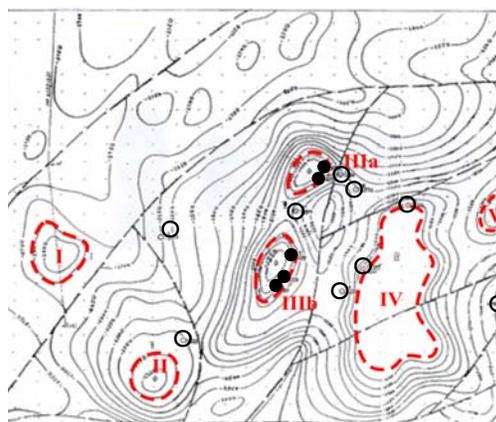
**Figure 2:** Latest seismic structural map (top of carboniferous sedimentary formation of Upper Jurassic). Conjectural outlines of positive structures: I, Kuchuc; II, Chuchuc; IIIa,b, East Buzakhur; IV, Karabay; V, Karayil. Contour lines show the top of the bed; black dashed lines are faults. Open circles are unproductive deep wells; solid circles are productive; dots are MT sites of the main grid.
