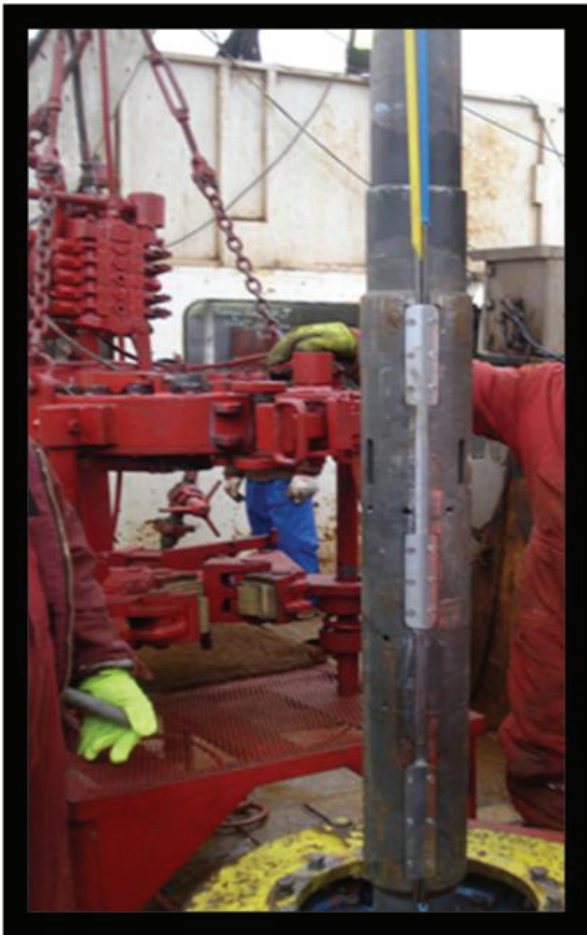
Figure 13: Sleeves and open hole Packers used in advanced Multi Stage Fracturing completions requires modifications to allow either single or multiple control line bypass for the Distributed Temperature Sensing (DTS) line and PDHMS lines. The photographs above show actual testing in the laboratory and field installation.
