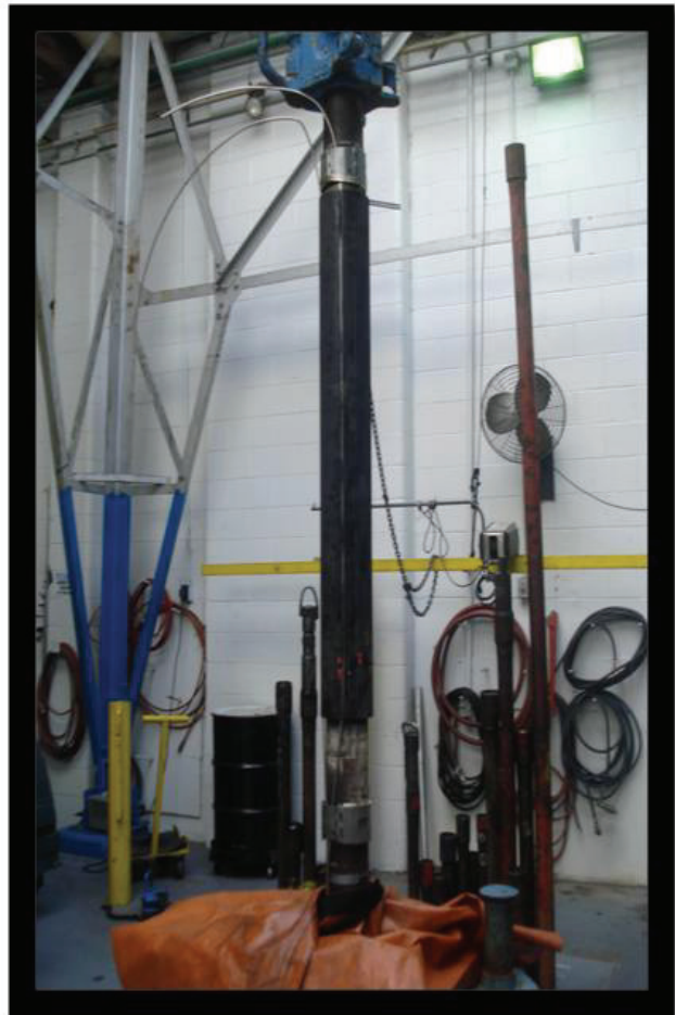
Figure 13: Sleeves and open hole Packers used in advanced Multi Stage Fracturing completions requires modifications to allow either single or multiple control line bypass for the Distributed Temperature Sensing (DTS) line and PDHMS lines. The photographs above show actual testing in the laboratory and field installation.
