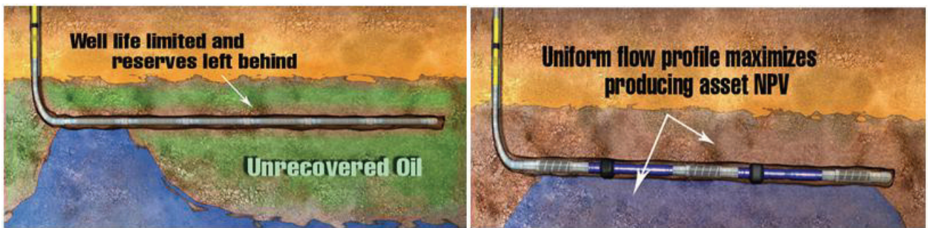
Figure 6: Comparison of reservoir drainage for natural flow reservoirs in standard open hole completion (upper) and reservoir optimized completions (lower), which use open hole packers (black) to segregate the lateral wellbore into three compartments. Hatched areas are inflow control devices adjusted to formation permeability profile along the wellbore.
