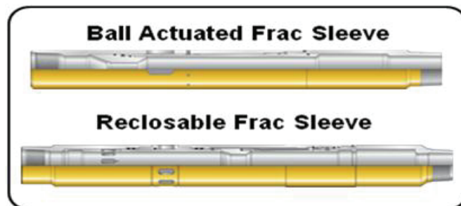
Figure 10: Frac sleeves can be divided into two types of Sleeves, namely a permanent locked open sleeve and re-closable sleeve.
