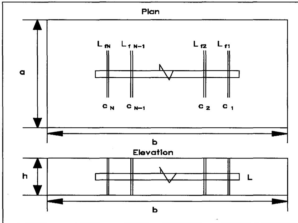
Figure 2. A Non-Fully Penetrating Horizontal Well Intersecting Natural Fractures
