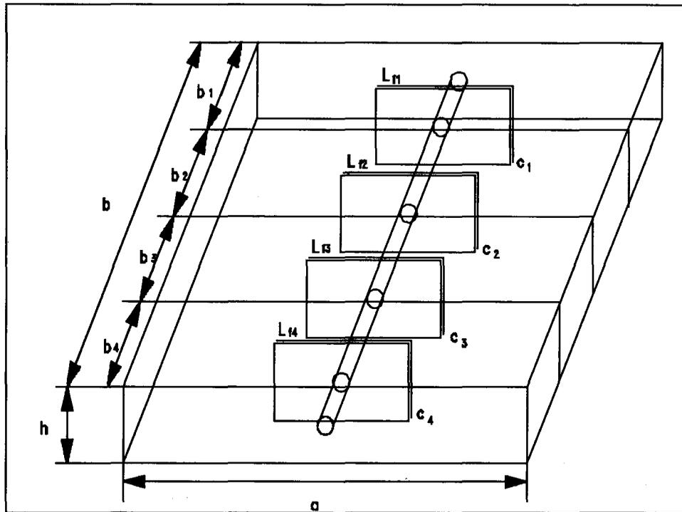
Figure 1. A Fully Penetrating Horizontal Well Intersecting Natural Fractures
