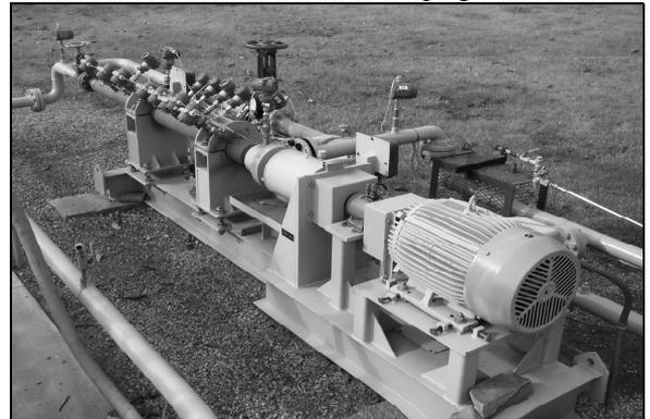
Figure 4: ESP test bench after modifications
