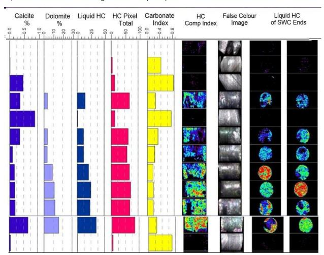
Results show the heterogeneity of the cores and the corresponding distribution of oils. The oil spectra were all similar to the OBM and the evidence indicated that OBM invasion was responsible for all of the oil identified. Analysis of the clay mineral polytypes was able to identify the K-rich clays that might influence the gamma log, it was clear these were not present in sufficient quantity to explain the high gamma values.
