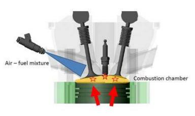
The specification which controls and limits the knock phenomenon is the Octane number. Octane is a comparative measurement carried out in the lab, with a specific engine.
