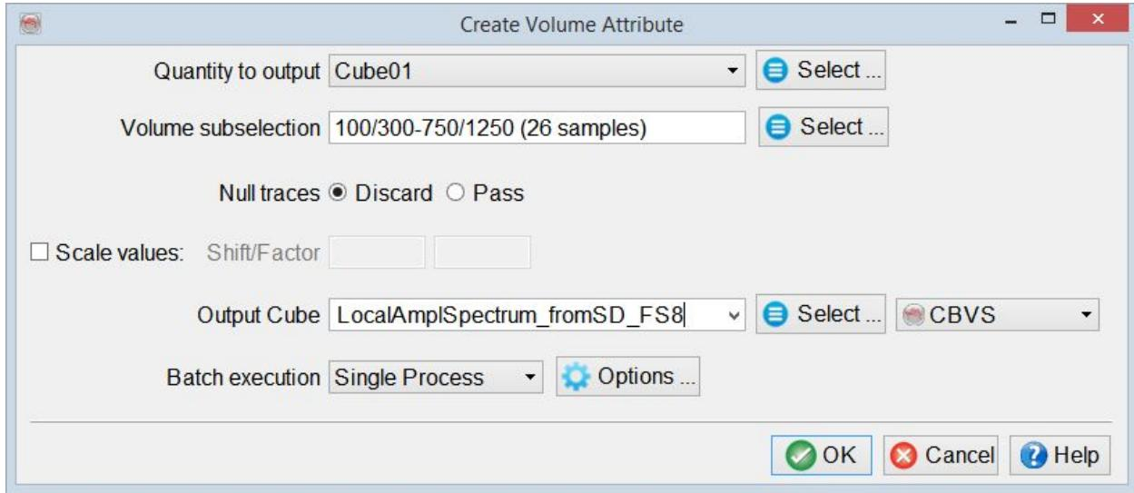
(optionally, limit Z range of the output cube via *Volume Subselection* for example, in this case it is limited to 0 - 100 ms as only samples 1-15 have actual data).
